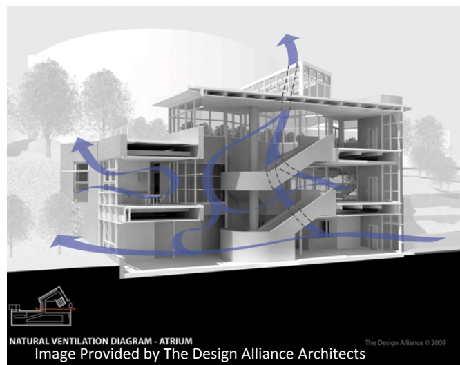
Figure 2 – Building section explaining the natural ventilation of the passively designed atrium.
